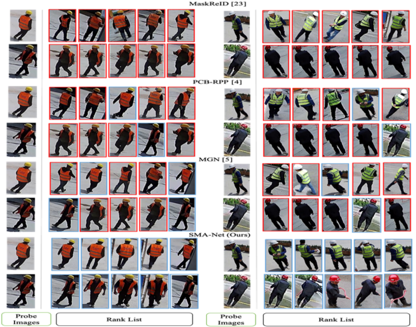
Fig.4. Examples of Re-ID results obtained by different methods. Red frames represent incorrect retrieval.
