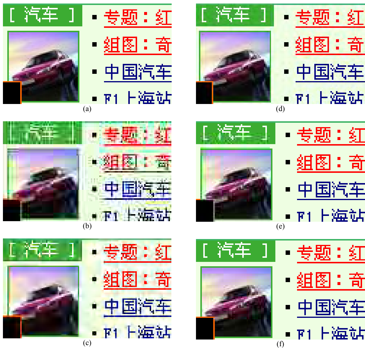
Fig. 10. Details of the sina image. (a) Original data, 1407KB. (b) JPEG, quality factor 17, 74KB, encoding 107ms, decoding 63ms. (c) JPEG 2000, compression ratio 19, 74KB, encoding 981ms, decoding 430ms. (d) DjVu, 260KB, run time unknown. (e) Our hybrid coding without intra-block segmentation, 66KB, encoding 104ms, decoding 24ms. (f) Our hybrid coding (with intra-block segmentation), 74KB, encoding 110ms, decoding 29ms.
